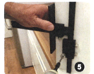
5 Flip tool to bottom of cabinet, position tool with Large Stop and T-square firmly against cabinet surface, and drill second set of holes
