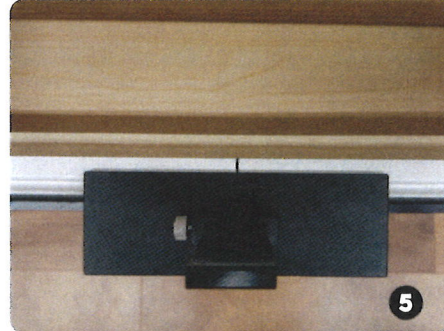
5 Line up notch on center of Large Stop with center mark at top of drawer then push tool flush against drawer face
