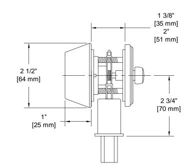
Door Prep: Cross Bore 2 1/8+, Edge Bore 1+, Latch Face 1 1/8+x 2 1/4+ Backset: 2 3/4+ Door Thickness: Standard Doors 1 3/8+to 2+ Cylinder: 6-Pin Removable Core Strike Plate: 2 3/4" Square Corner Standard Bolt: 1" Throw, Nickel Plated ANSI/BHMA: A156.5 Grade 2
