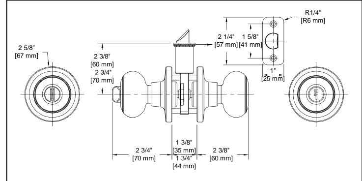
Door Prep: Cross Bore 2 1/8+, Edge Bore 1+, Mortise Latch Face 1+x 2 1/4+, Optional Drive In Latch 1" Diameter Drilled Hole
