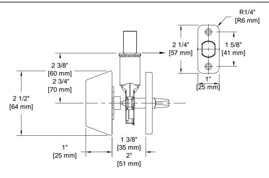
Door Prep: Cross Bore 2 1/8+, Edge Bore 1+, Mortise Latch Face 1+x 2 1/4+, Optional Drive In Latch 1" Diameter Drilled Hole
