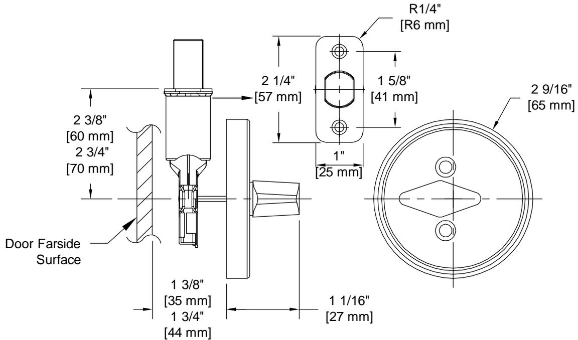
**Door Prep:** Cross Bore 2 1/8+, Edge Bore 1+, Mortise Latch Face 1+x 2 1/4+, Optional Drive In Latch 1" Diameter Drilled Hole
