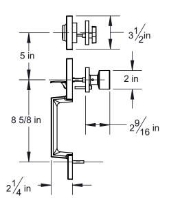
Door Prep: Cross Bore 2 1/8", Center To Center 5 1/2", Edge Bore 1", Mortise Latch Face 1" X 2 1/4" X 1/4"
