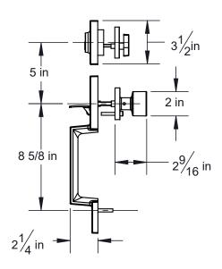
Door Prep: Cross Bore 2 1/8", Center To Center 5 1/2", Edge Bore 1", Mortise Latch Face 1" X 2 1/4" X 1/4" Radius,
