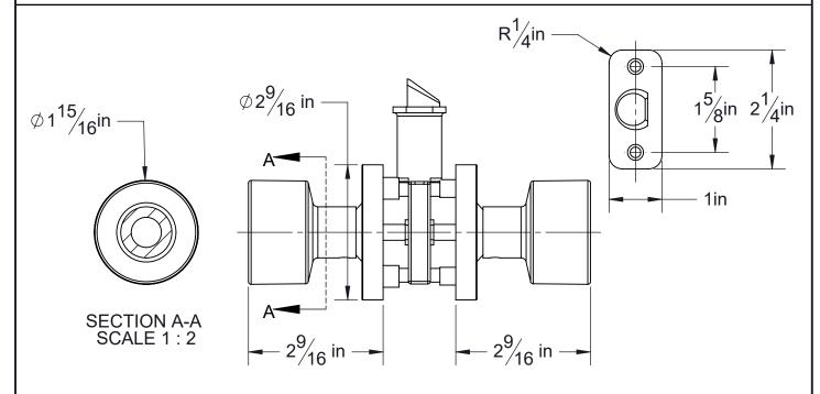
Door Prep: Cross Bore 2 1/8", Edge Bore 1", Mortise Latch Face 1" x 2 1/4", Optional Drive In Latch 1" Diameter Drilled
