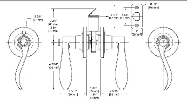
Door Prep: Cross Bore 2 1/8+, Edge Bore 1+, Mortise Latch Face 1+x 2 1/4+, Optional Drive In Latch 1" Diameter Drilled Hole Latches: Ships With Mortise Latch As Shown Above. Optional Drive In Or UL10C Fire Rated Latches Available
