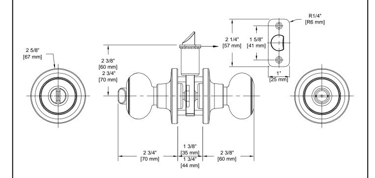
Door Prep: Cross Bore 2 1/8+, Edge Bore 1+, Mortise Latch Face 1+x 2 1/4+, Optional Drive In Latch 1" Diameter Drilled Hole
