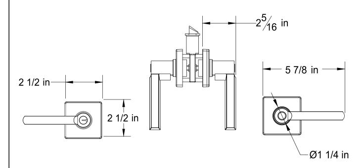
Door Prep: Cross Bore 2 1/8", Edge Bore 1", Mortise Latch Face 1" X 2 1/4", Optional Drive In Latch 1" Diameter Drilled Bore
