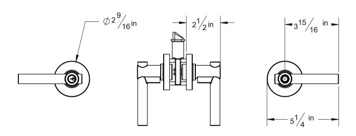
Door Prep: Cross Bore 2 1/8", Edge Bore 1", Mortise Latch Face 1" X 2 1/4", Optional Drive In Latch 1" Diameter Drilled Bore
