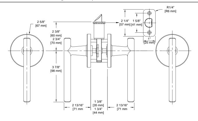
Door Prep: Cross Bore 2 1/8+, Edge Bore 1+, Mortise Latch Face 1+x 2 1/4+, Optional Drive In Latch 1" Diameter Drilled Hole
