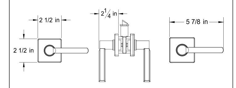
Door Prep: Cross Bore 2 1/8+, Edge Bore 1+, Mortise Latch Face 1+x 2 1/4+, Optional Drive In Latch 1" Diameter Drilled Hole
