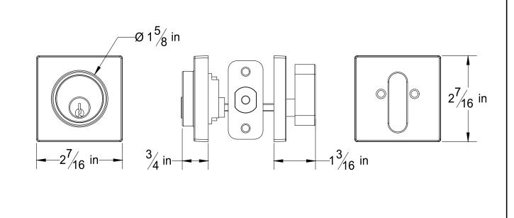
**Door Prep:** Cross Bore 2 1/8", Edge Bore 1", Mortise Latch Face 1" x 2 1/4", Optional Drive In Latch 1" Diameter Drilled Hole **Latches:** Ships With Mortise Latch As Shown Above. Optional Drive In Or UL10C Fire Rated Latches Available **Backset:** Adjustable Latch to 2 3/8" or 2 3/4"
