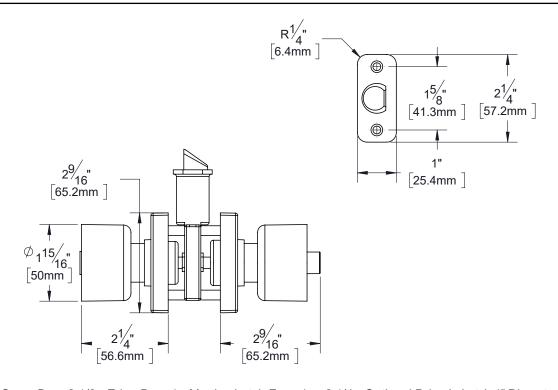
Door Prep: Cross Bore 2 1/8+, Edge Bore 1+, Mortise Latch Face 1+x 2 1/4+, Optional Drive In Latch 1" Diameter Drilled Hole
