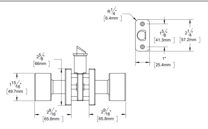
Door Prep: Cross Bore 2 1/8", Edge Bore 1", Mortise Latch Face 1" x 2 1/4", Optional Drive In Latch 1" Diameter Drilled Hole
