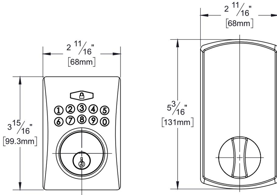
**Door Prep:** Cross Bore 2 1/8", Edge Bore 1", Latch Face 1" x 2 1/4"
