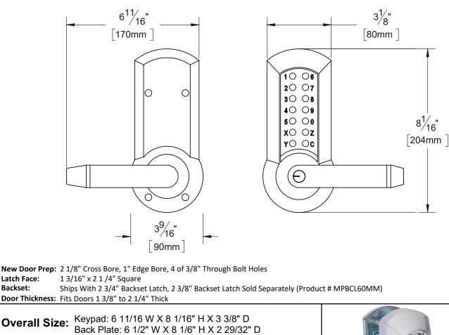
Material: Die Cast Zinc Body, Stainless Steel Push Buttons and Latch Bolt
