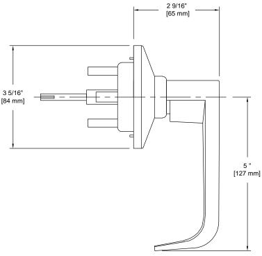
Door Thickness: Standard Doors 1 3/8" To 1 3/4" With Available Extension Kit Fits Doors 2 1/4" Cylinder: Solid brass 6-Pin Removable Core Schlage "SC 1 Keyway"
