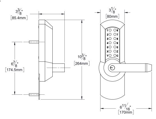
New Door Prep: 2 1/8" Cross Bore, 4 of 3/8" Through Bolt Holes
