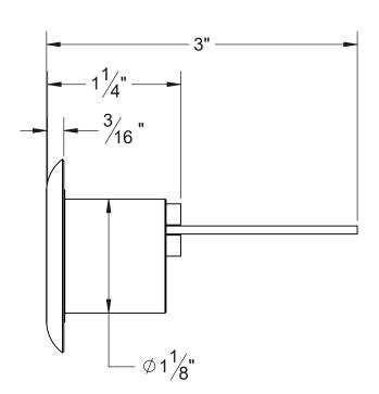
**Door Thickness:** Standard Doors 1 3/4" - 2 1/2" **Cylinder:** Solid Brass 5-Pin Schlage "SC 1 Keyway"
