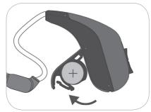
To power on, insert battery (+ side up) as shown and close the door. To power off, open the battery door.
