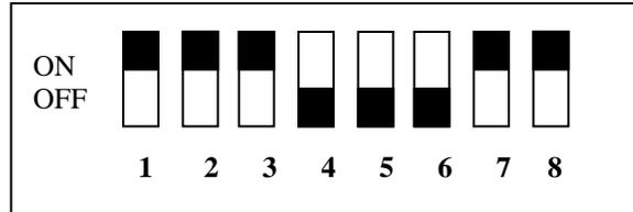
DB Sensor settings (smaller unit) for dip switches 1 thru 6 are set at the factory and only need to be changed if your neighbor has a DB100 or DB200. The 8 dip switches should be set as follows:
