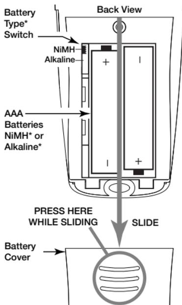
**\*NOTE: If using rechargeable NiMH AAA batteries, the battery switch MUST be switched to the NiMH position to allow charging!**
