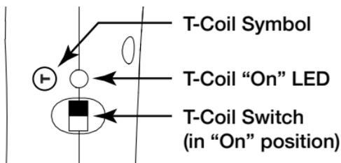
**Note:** For best performance when using the T-coil feature, the Pocketalker must be in a **vertical** orientation. This ensures the best magnetic coupling to the loop system. When the T-coil switch on the Pocketalker is enabled, the Pocketalker disables the microphone input.
