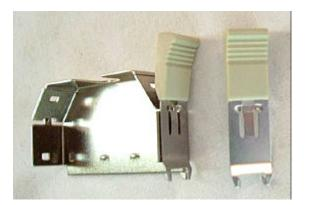
The clips snap over a small tab on the sides of the outer shroud. With respect to this illustration, you would place the clip against the shroud and up a little, then as you slide the clip down the side, the tab would come up through the center, and the longer tab on the clip will eventually snap. When both clips have been snapped on, the outer shroud can then be snapped to the inner shroud around the connector.
