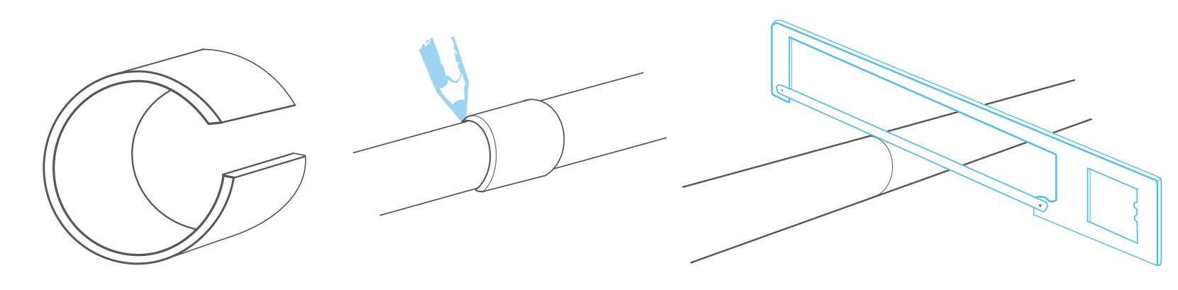
Use the cutting clip to trace around the legs 'C' at the calculated length attained from using the Leg Length Table. Then with the hacksaw ensure the cut follows the line drawn. Take care so that all the legs are of equal length.
