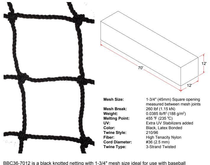
BBC36-7012 is a black knotted netting with 1-3/4" mesh size ideal for use with baseball batting cages. Netting comprized of high tenacity fiber resistant to abrasion and light weight. All perimeters of netting shall be sewn together and bound to a 3/8" polypropylene rope. Netting shall be sufficient size to allow for approximately 1' of netting to lay on the floor when caged is beign used.
