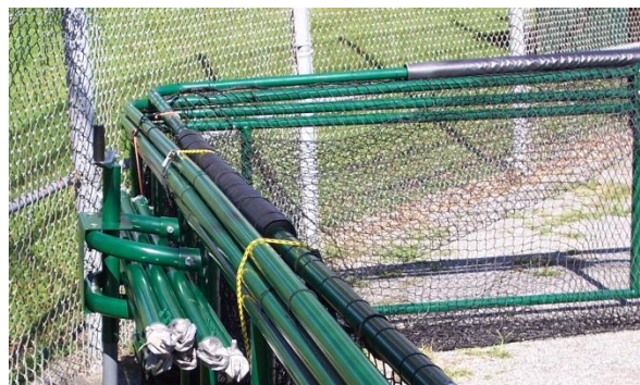
Strut pipe clamps (5) to be store in between jack bracket (13).
