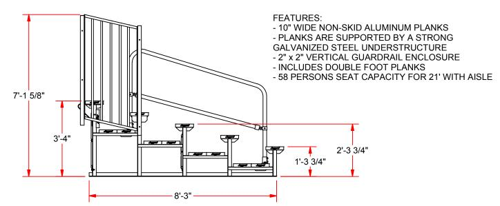
5 ROW 21 FT GUARD RAIL W/ AISLE AND HANDRAIL
