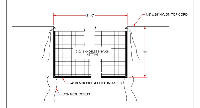
This net shall be for use on any Badminton Systems. Net shall meet the requirements set forth by all governing bodies for Badminton. Net shall be 21' long x 30" high with a top cable of 1/8" nylon cord. Constructed with a 1 1/2" white top band and 3/4" black side & bottom tapes. All corners shall have grommets and control cords to help position the net.
