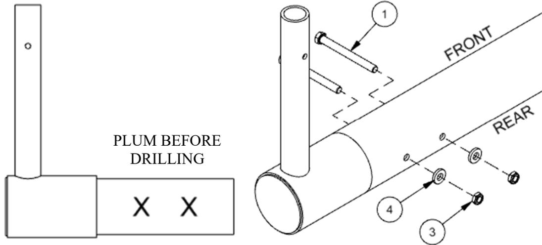
Insert the end fitting in crossbar and loosely install the appropriate hardware. Verify that the vertical member is square to the crossbar and plumb.
