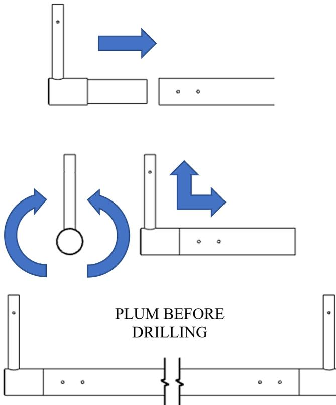
Remove the end fitting and drill the marked holes. Start with a 3/16” bit, then a 3/8” bit and finally a ½” bit.
