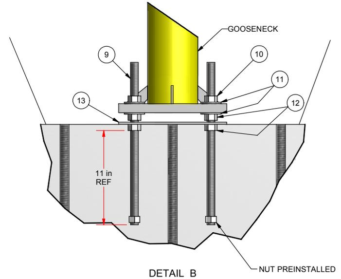
IT IS STRONGLY RECOMMENDED THAT THE POURED FOOTING BE REINFORCED WITH A MINIMUM OF 6 PIECES OF 3/4" x 66" RE-BAR
