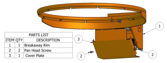
Figure 5-1: Cover plate removal/installation.
