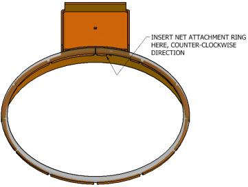
Figure 5-4: Insert Net Ring in counter-clockwise direction.
