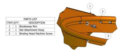
Figure 5-6: Screw net attachment ring to rim.
