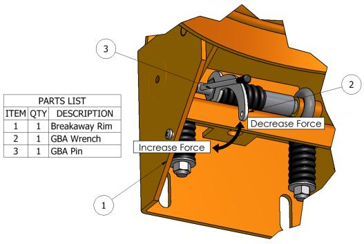
Figure 6-1: Adjust spring tension.
