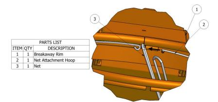
Figure 5-5: Pass net attachment ring through long net loops.
