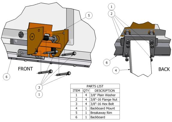
Figure 5-2: Attach rim to backboard.
