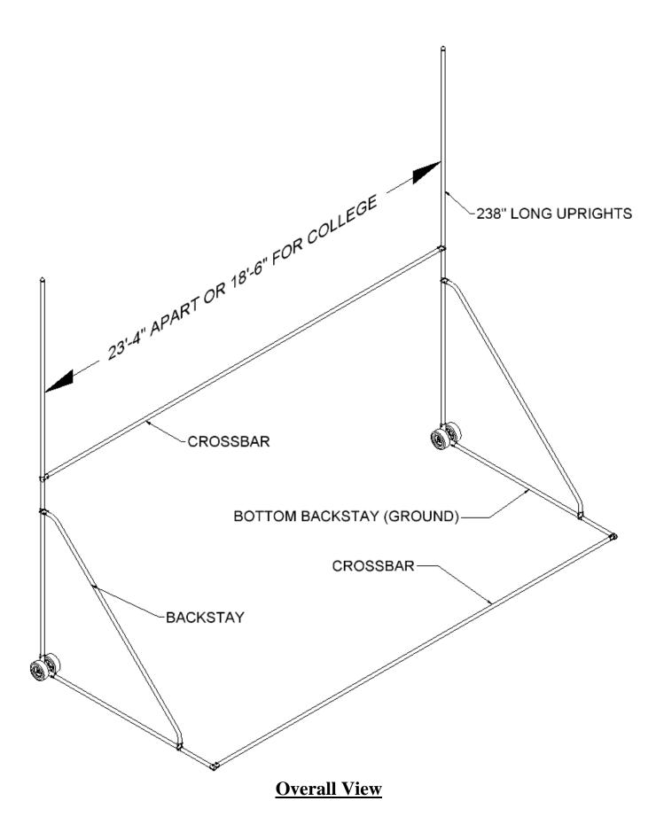
1. Place the uprights on ground, parallel to each other, 23'-4" apart (18'-6" for college). Ends of pipes with two holes spaced 8" apart are going to be at the bottom of goal.
