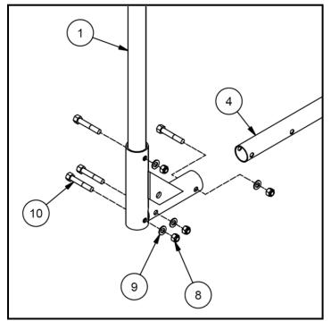
4. Insert bottom backstay pipes into wheel assembly weldment. Assemble hex bolts, washers and nuts as shown above, tighten nuts fully. Allow these pipes to lay on the ground as they are being assemble.
