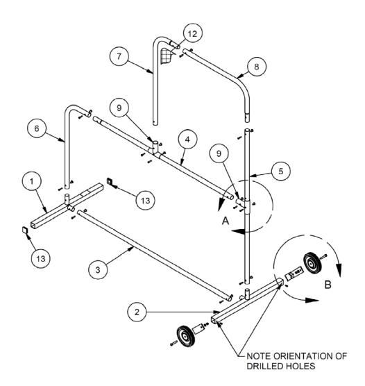
Figure 2 Wheel Orientation
