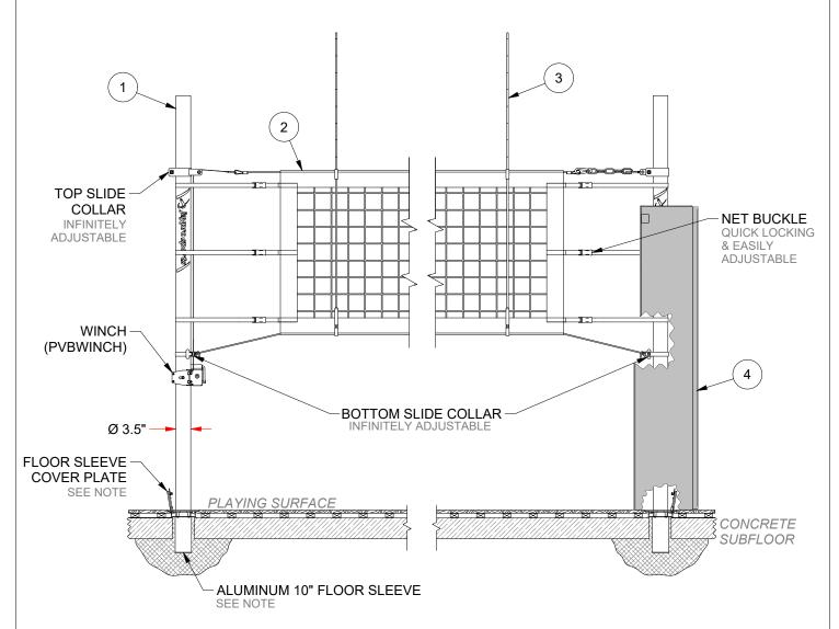
NOTE: FLOOR SLEEVES REQUIRED TO INSTALL SYSTEM. FLOOR SLEEVE COVER PLATES AVAILABLE IN BRASS AND CHROME FINISHES. FLOOR SLEEVES & COVER PLATES SOLD SEPARATELY.
