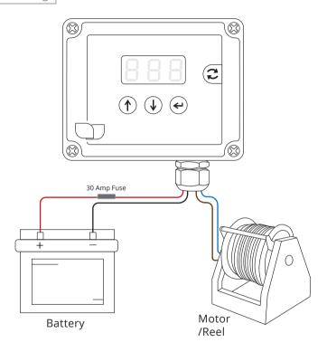
Connect the Reel Winder in accordance with this diagram. NOTE: only fit the fuse once all connections are made.
