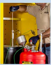
Use drum pumps to safely transfer hand sanitizer into intermediate containers. Includes pre-assembled bonding and grounding clamps to help control static discharge.
