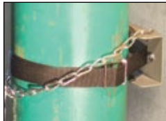
Secure gas cylinders to wall or bench to prevent dangerous tipping.
