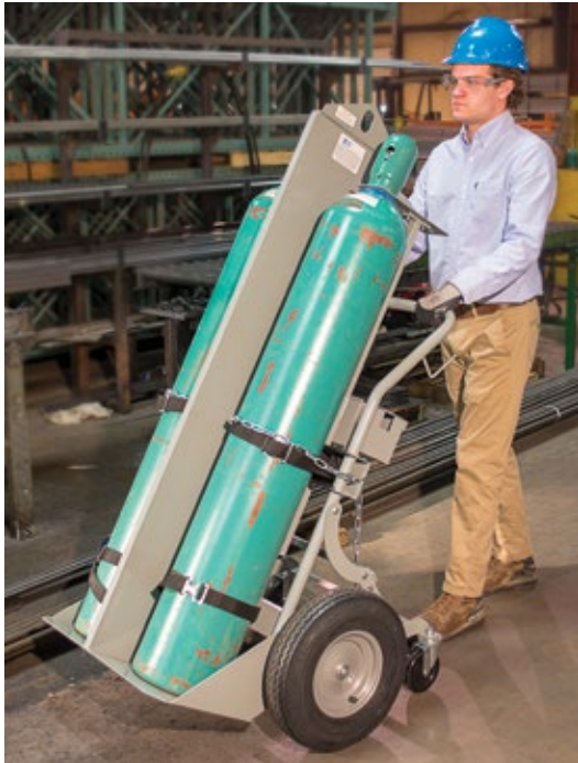
Firewalls exceed minimum separation requirements for extended storage of fuels and oxidizers in close proximity.
