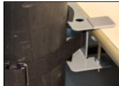
Secure gas cylinders to wall or bench to prevent dangerous tipping.
