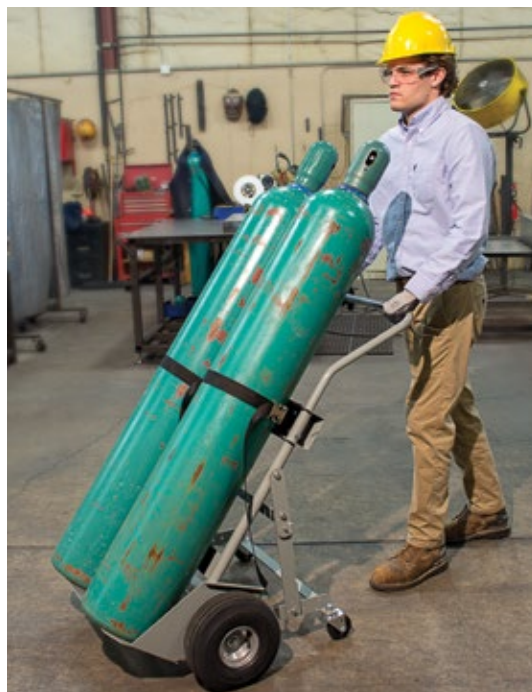
Double cylinder hand truck holds gas cylinders in place independently for improved safety.
