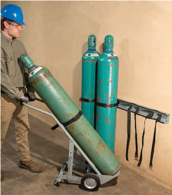
All compressed gas-cylinders in service or in storage at user locations should be secured to prevent falling or rolling.
