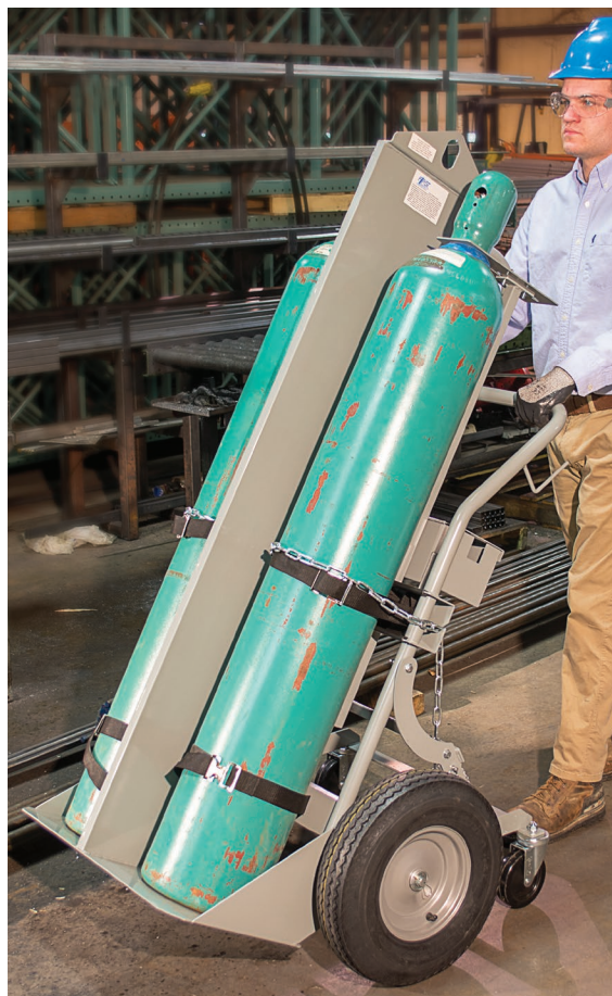
Firewalls exceed minimum separation requirements for extended storage of fuels and oxidizers in close proximity.
