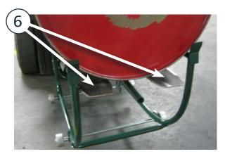
Lift truck forks fully supporting drum cradle and drum.
