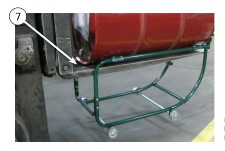
Maintain adequate clearance between lift truck forks, mast and any fittings installed in the head of the drum.
