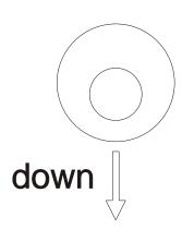
Bushings must be installed with offset hole down and centered in the 6 o'clock position.
