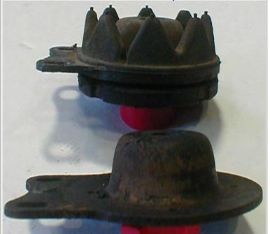
Insert bushing 2698 so the flange is on top of the differential case as pictured below.
