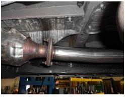
1) Place the right side inlet pipe **#86461M** and left side **#86462M** into position and fasten the flanged connections together using the bolts removed in step 3 above.
