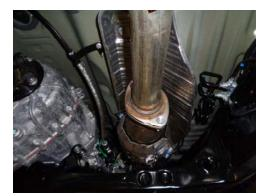
3) Support the muffler with a stand, then using a 14mm socket; unbolt the 4 bolts at the two front flanged connections. Separate the wire hangers in front and rear of the muffler from the rubber mounts on the vehicle. Remove the muffler inlet pipe assembly and set aside. Save the 4 factory bolts, they will be reused in Installation step 1.
