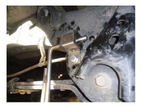
6) Align the hole in the **HA602** rubber mount with the upper hole in the front leaf spring perch. Use the supplied 3/8" Bolt, Nut and washers to mount the hanger in place. Tighten securely.
