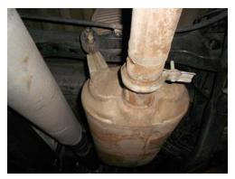
2) Using a 12mm socket, unbolt the tailpipe connection where it exits the muffler. Separate the wire hanger on the tailpipe from the rubber mount on the vehicle. Remove the tailpipe and set aside.
