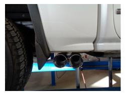
7) Adjust the position of all pipes and muffler to provide a satisfactory fit. A minimum 3/4" clearance around all parts of the system must be maintained; while also keeping suspension travel and vibration in mind.
