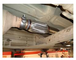
1) Place inlet pipe assembly **#26687M** into position onto the ball connection behind the catalytic converter. Reinstall the clamp onto the ball connection and tighten enough to hold, but still allow for a small amount of adjustment. Connect the hanger on the pipe to the rubber mount on the vehicle.
