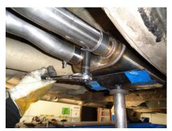
5) Place a supplied 2-1/2" clamp onto each muffler outlet. Place the exit pipe assembly **#86465M** up into position and slide into both muffler outlets approximately 2". Use a stand to support the outer end of the assembly. Tighten the clamps just enough to hold in position.
