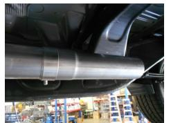
2) If installing the system on a Crew Cab truck with a 6.5' bed, place extension pipe **#TB700M** onto the back of the **#26687M** inlet pipe, place a provided clamp onto the slip-fit and tighten enough to hold in position. This extension pipe will not be used on Double Cab or Crew Cab-5.5' bed models.
