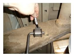
6) Adjust the exit pipe so that the tips are the desired distance from the body, then rotate the **HA572** hanger so that it lays flat against the inside of the vehicle frame and use a center punch to mark the center of the two holes on the frame. Rotate the hanger out of the way and drill each mark using a <sup>1</sup>/<sub>4</sub>" drill bit. Use the two 5/16" thread cutting bolts to secure the hanger to the frame. Tighten securely.
