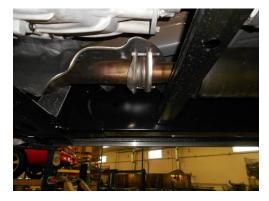
3) Support the muffler with a stand and remove the two bolts at the front flange connection. Now, with the help of an assistant, slide the exhaust system to the rear to disengage the rubber hangers from the mounts on the vehicle. Once free, the assembly can be removed by working it forward over the rear axle (If you are working on the ground it may be easier to cut the tailpipe off at the rear of the muffler to simplify removal).
