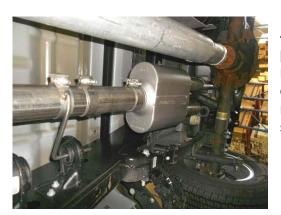
4) Slide the inlet hanger #490HA over the back of the inlet pipe and insert the hanger into the factory rubber mount. Do not tighten this clamp yet. Then place the inlet of the muffler onto the back of inlet pipe and support with a stand. Level the muffler and tighten the clamp at the inlet enough to hold, but still allow for adjustment.
