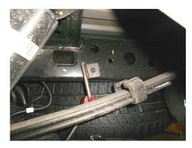
1) Mount the left rear tailpipe hanger bracket **#226HA** to the frame on the driver's side of the vehicle. Place the included 3/8 x 3.50" bolt thru the HA226 hanger and into the hole indicated in the photo. On the inside of the frame, place the HA226 back-up plate over the bolt followed by a flat washer, lock washer and nut. Using two 9/16" wrenches tighten firmly (Do not over tighten).
