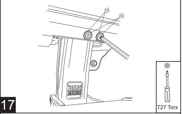
Using a T27 Torx driver torque bolts to 6 ft-lbs.
