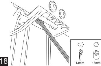
**All Linkages:** Slide linkage over pre threaded bolts. Using a T27 Torx driver start torx bolts and washers. Snug bolts but do not tighten. Replace bolts from step 15 if present.
