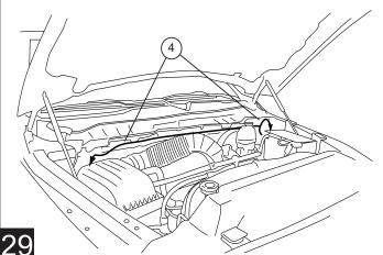
Using a 4mm hex key torque bolts to 36 in-lbs. **See page 2 for motor installation instructions.**
