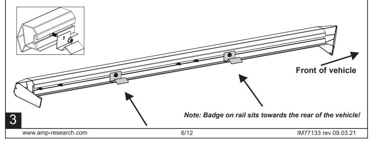
Adjust bolts and slide over brackets. Use supplied flange nuts and attach rail to brackets.
