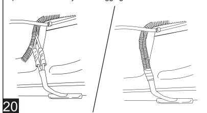
Reinstall Fuses from Powerstep Wire Harness.
