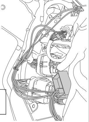
NOTE: Bundle Pin 3 & 4 wires and Pin 8 & 9 wire together in posi tap since rear doors are not present. Failure to do so will result in incomplete door signals.
