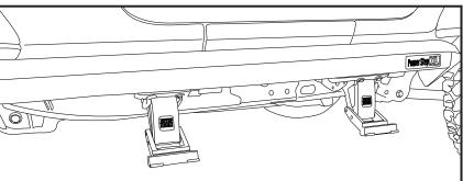
Install provided spacer (2019) and M6 bolt (11) into upper mount as shown on both the drive and idler linkages. Do not tighten.
