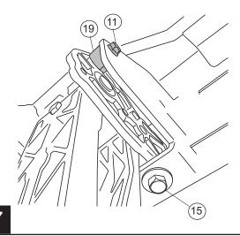
Slide mounting T-nut into position. Center board in rail pocket. Tighten fasteners to 10 ft-lb
