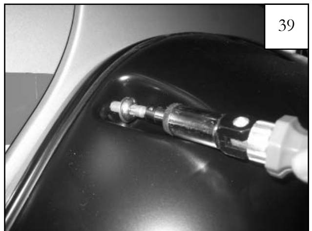
Start Screws/Washers through pocket holes in Outer Flare and into "U" Nuts installed in Step 17 (8 places). Do not tighten.
