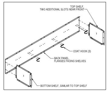
Step 2: Turn the back panel on its back with the shelves pointing upward. Attach the first side panel, the left rear leg, and two compartment dividers to the assembly from Step 1. Attach an additional three coat hooks to the first side panel.
