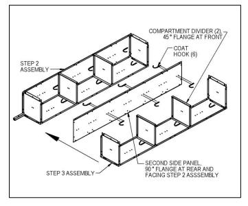
**Step 5:** Attach the third top shelf, the third bottom shelf, and an additional three coat hooks to the third back panel as in steps 1 and 3.
