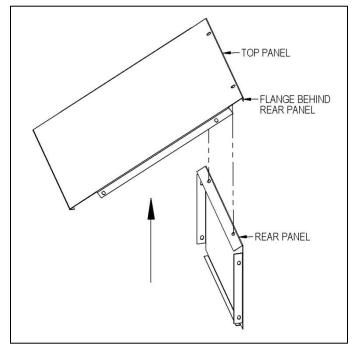
Step 2: Assemble the side panels to the top panel and rear panel with #10 - 24 x 3/8" long slotless screws and #10 nuts (provided)
